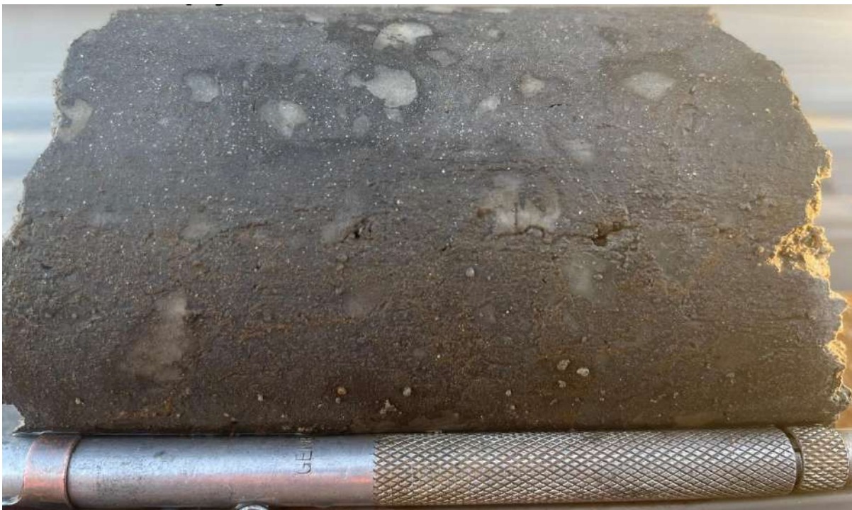
Image 3. CDX0004, 91m, milled breccia with quartz clasts in sulphidic matrix. High grade niobium zone of 9m at 1% Nb 2 O 5 and 2.3% TREO from 84m.
