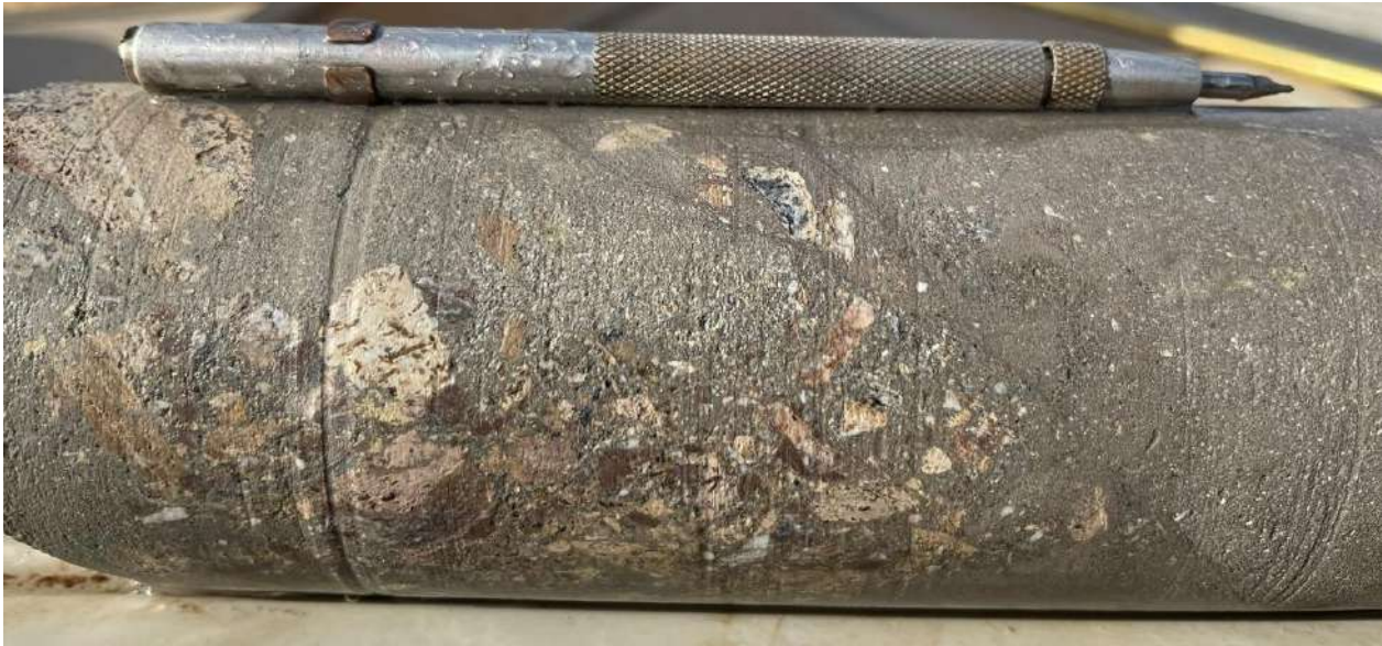
Image 2. CDX0011 130m, fault breccia with dark sulphidic high grade rare earths matrix.
