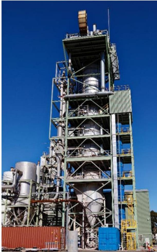
Above: The Calix Flash Calciner and Electric Pilot Scale Plant (BATMn Reactor)
