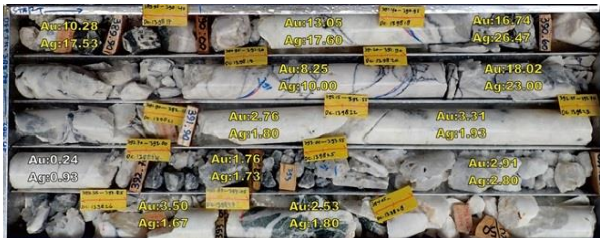
Figure 3. Drill core from Talang Santo 3 Main Vein (DDH-577 - 4.45m @ 8.43 g/t Au and 12.9 g/t Ag from 389.6m, including: 2.95m @ 11.6 g/t Au and 18.5 g/t Ag from 389.6m).
