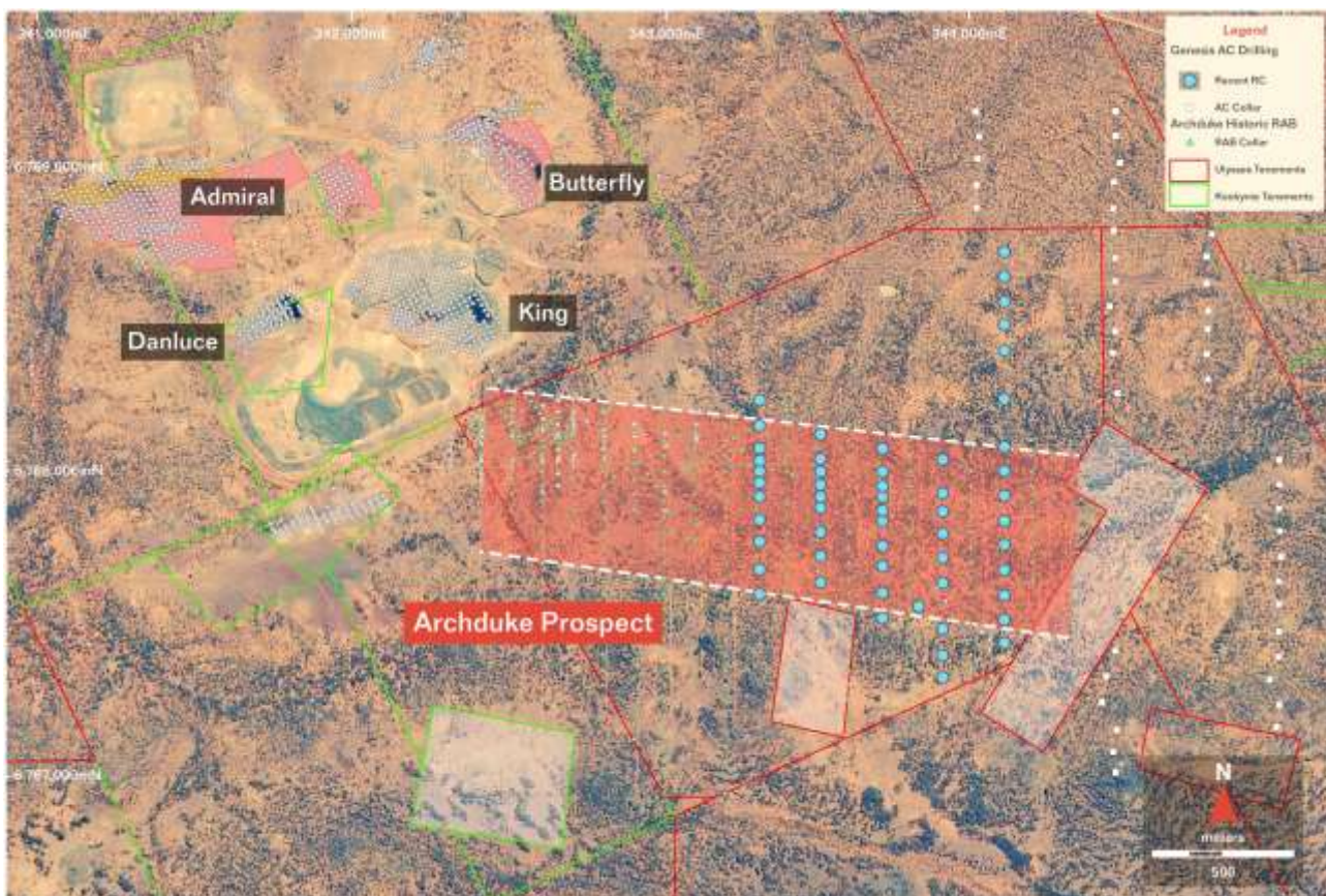
Figure 2. Archduke location with recent aircore drilling. Collar locations highlighted by light blue circles.
