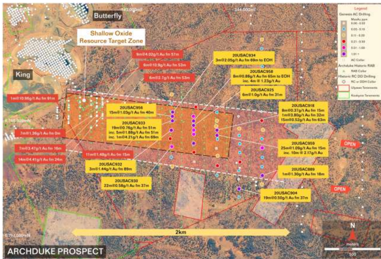
Figure 3. Recent aircore drilling results highlighted in yellow boxes.
