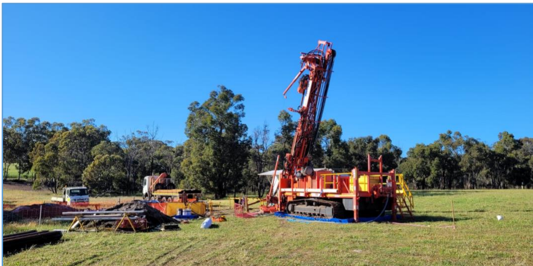
Figure 1. Diamond drill rig in operation at the Sovereign Project, WA. Drilling is designed to understand the geometry and extent of the intrusion at depth including the prospective ultramafic rocks (serpentinite).
