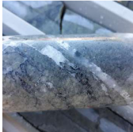
Photo 5. SNDD002 from 446m altered and veined (quartz) felsic volcanics with minor disseminated pyrite
