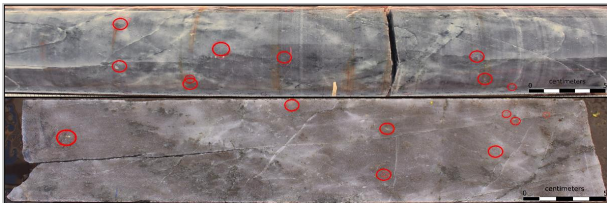
Photo 1: BBDD0130; Tura Steep Lode with visible gold circled in red Top: Tura full HQ core from 401.77m to 402.2m; Bottom: Tura half HQ core from 401.69m to 402.00m
