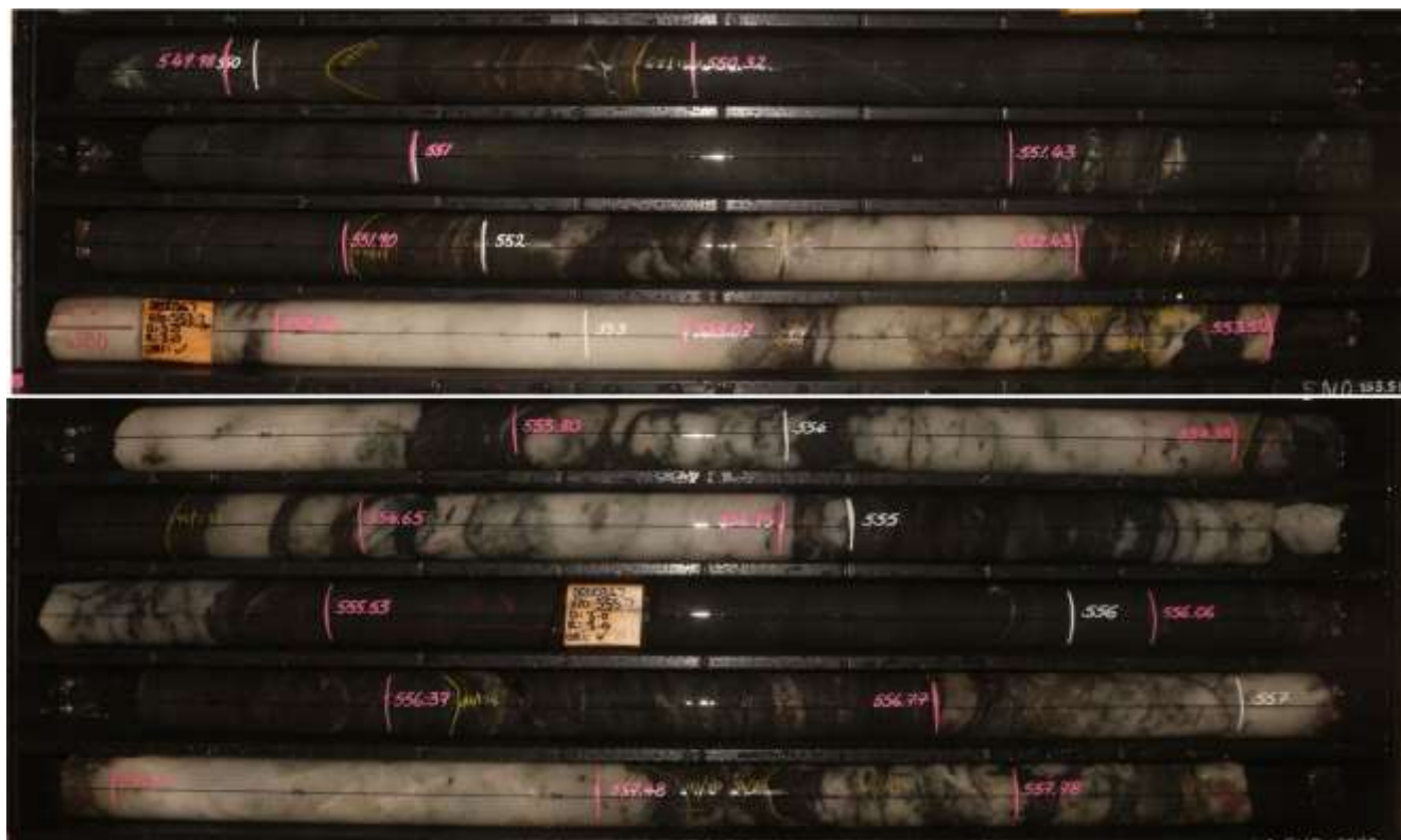
Figure 4: DRDD367 ext. Interval comprises dominantly milky quartz veining with associated biotite shearing and boudinaged quartz veinlets. +25 specks of visible gold occurring at the end of the second zone. Fracture fill/semi-cataclastic 10% pyrrhotite and trace chalcopyrite forming within the quartz vein. Pyrrhotite and chalcopyrite disseminated and forming as stringer veins within the biotite shear. Assays pending
