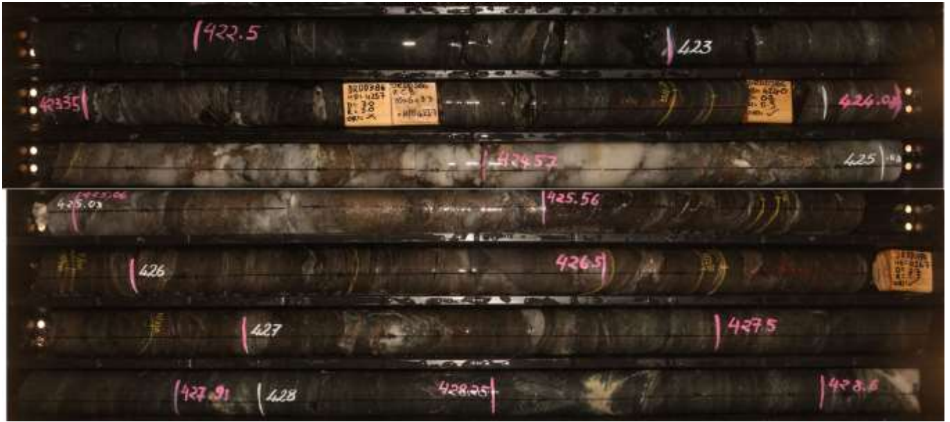
Figure 2: DRDD386 Interval comprised of a 1.5m milky (50%) and smokey quartz vein with associated biotite shearing on margins. +50 specks of visible gold observed within the quartz vein, evenly distributed throughout the vein. 15% pyrrhotite and trace chalcopyrite occurs as cataclastic and fracture fill within the vein and as stringer veins within the shear. Assays pending
